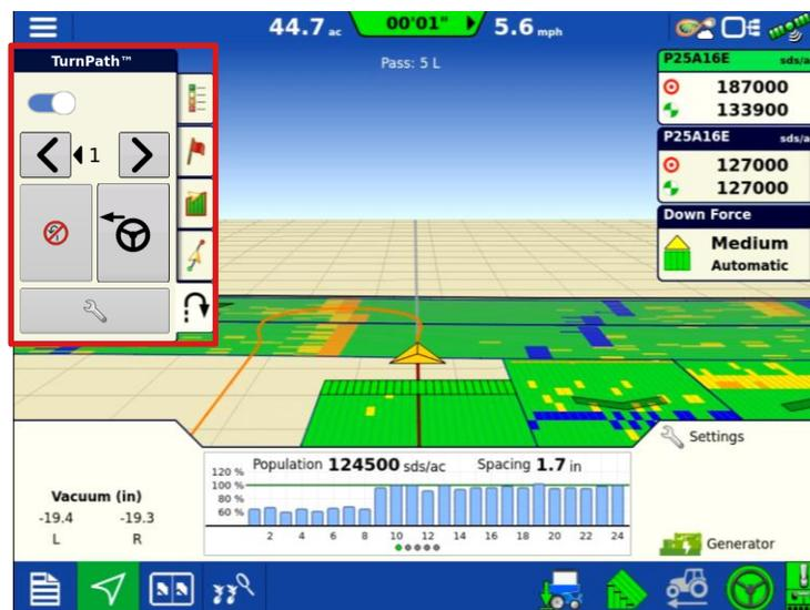
Figure 1 – TurnPath™ for automatically autosteering through end of row turns. Unlock Required
